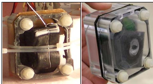
Figure 1: a) Left: MFC with the cathode half-cell open-to-air, b) Right: MFC with the closed chamber cathode half cell
