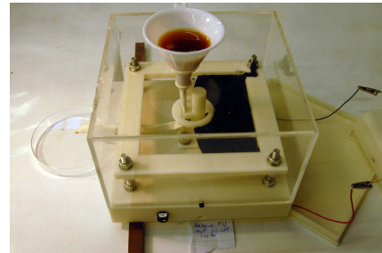
Fig. 5. Photograph of the DEA sphincter that was actuated using the MFC capacitor.
