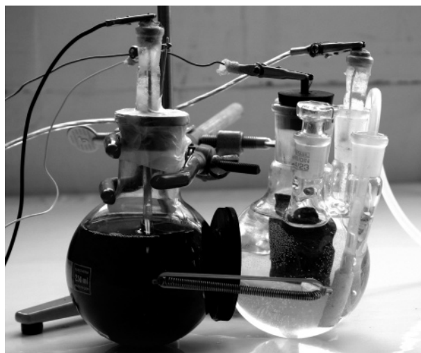
FIGURE 4. Photograph of the batch-type microbial fuel cell setup. Cathode and anode compartment were equipped with reference electrodes. The cathode compartment was purged with air by means of a fish pump and a diffuser. Both compartments were stirred.
