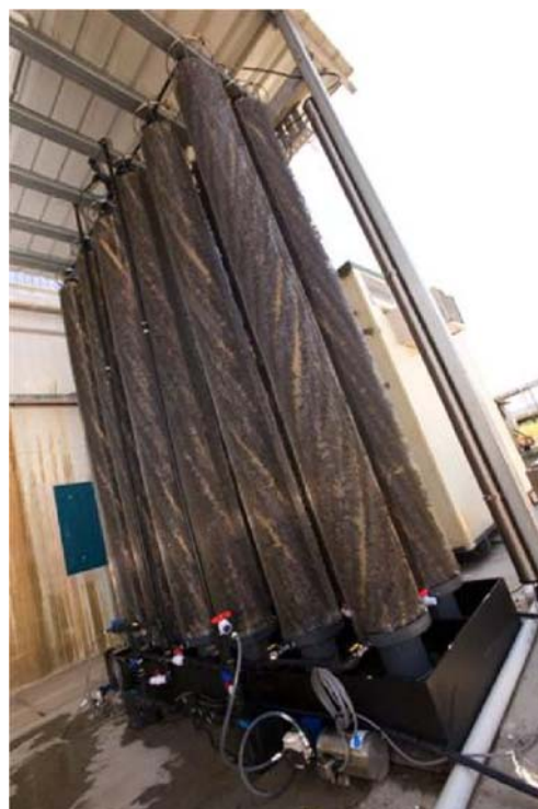
Fig. 3 Tubular microbial fuel cells tested for power production using wastewater produced at Foster's brewery in Yatala, Australia ( www.microbialfuelcell.org )
